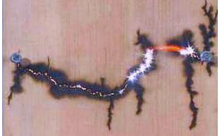
Active partial insulation failure due to tracking.
